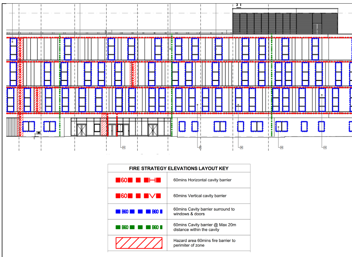
Figure 5 – Extract from drawing number HLM-SZ-SL-EL-572-001 showing cavity barrier provision
