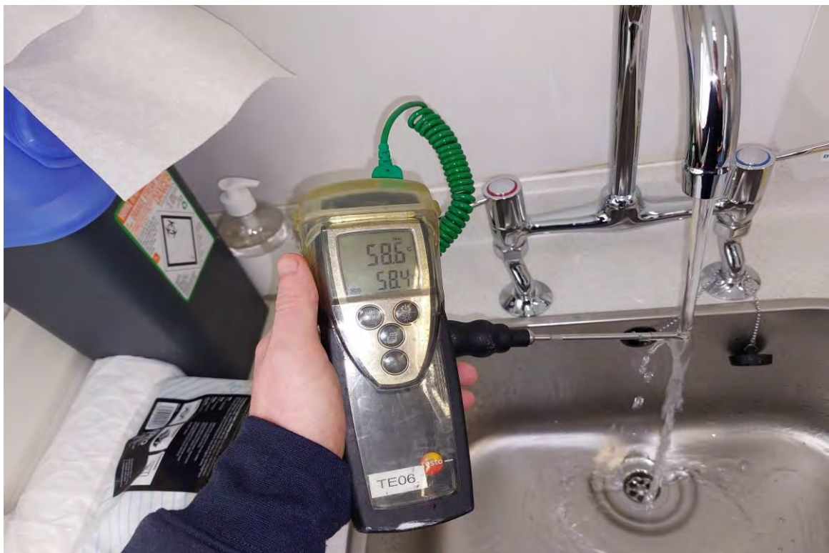
Extension Consultant Room 3 Sink - Hot Water Outlet Temperature Satisfactory
