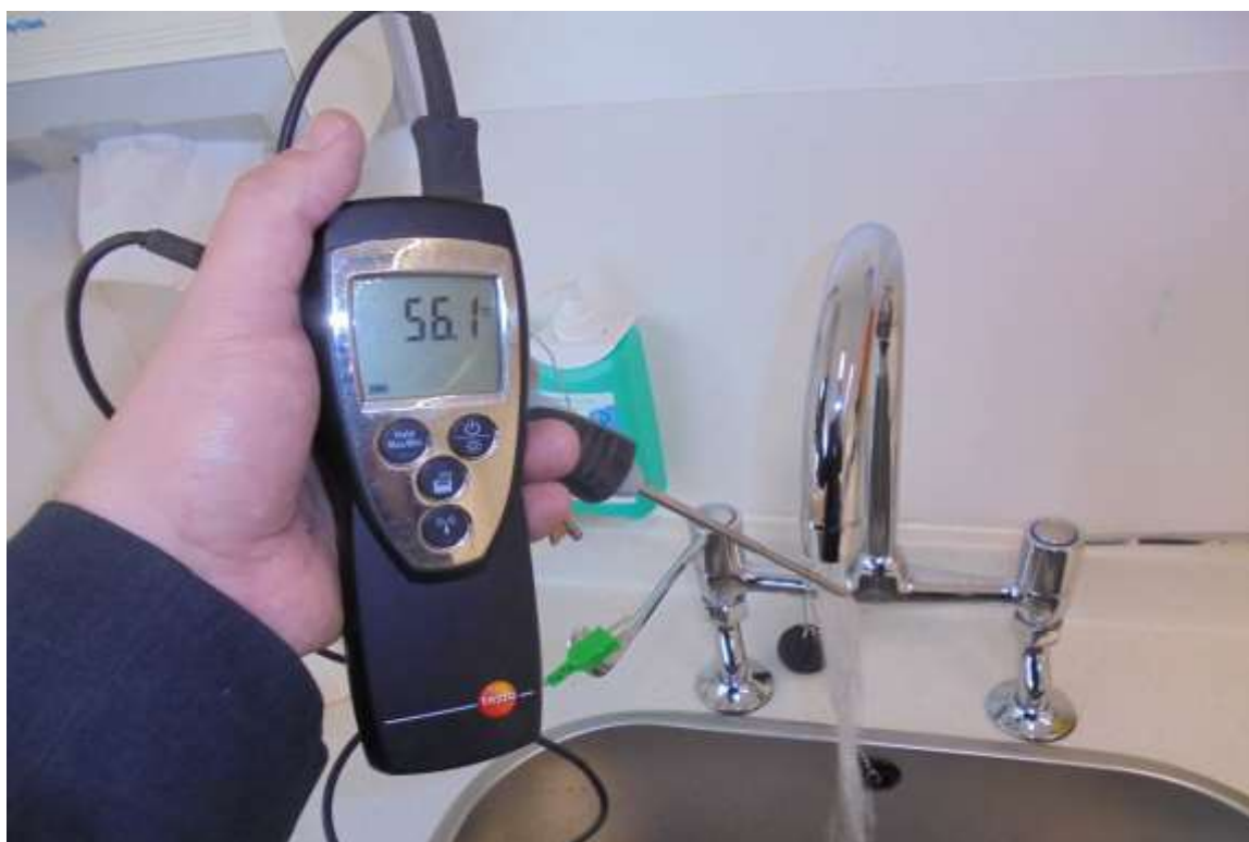
Extension Consultant Room 2 Sink - Hot Water Outlet Temperature Satisfactory
