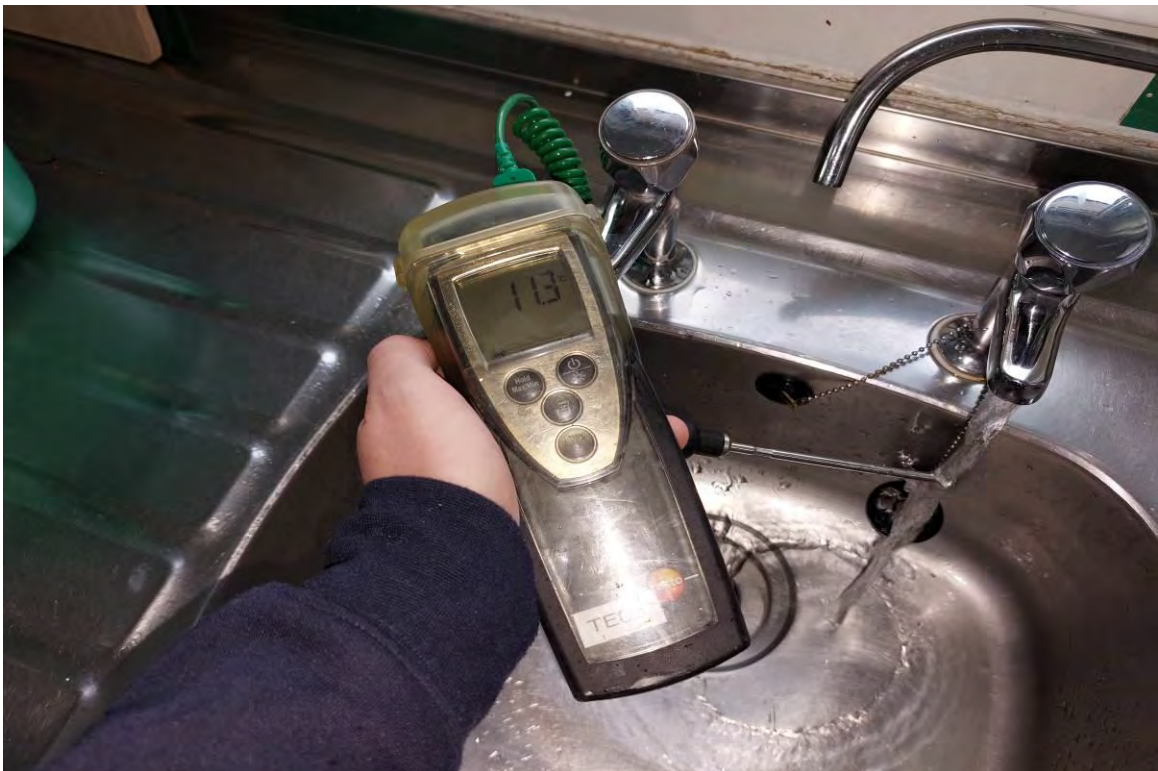
1st Floor Staff Room Sink – Cold Water Outlet Temperature Satisfactory
